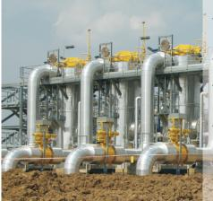
service access to candle filter cartridges through bayonet closure with hydraulic quick opening system
