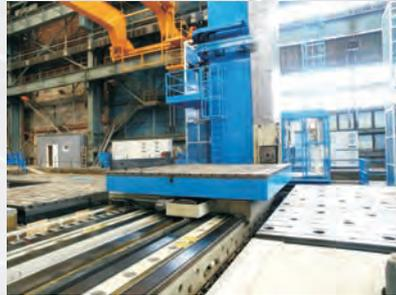
*CNC - Fräsbohrmaschine*
