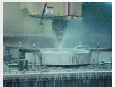
Drilling of heat exchanger tube sheet
