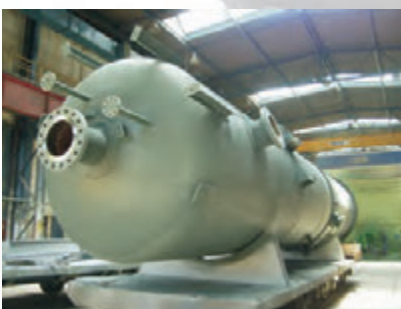
Pressure vessel for petrochemical plant
