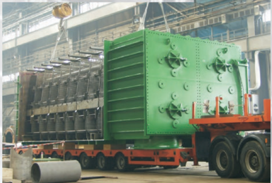
Assembly and transport of steam condenser
