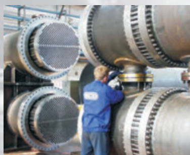
Trial assembly test of shell & tube heat exchangers installed as stacked unit
