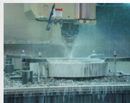
Drilling of heat exchanger tube sheet
