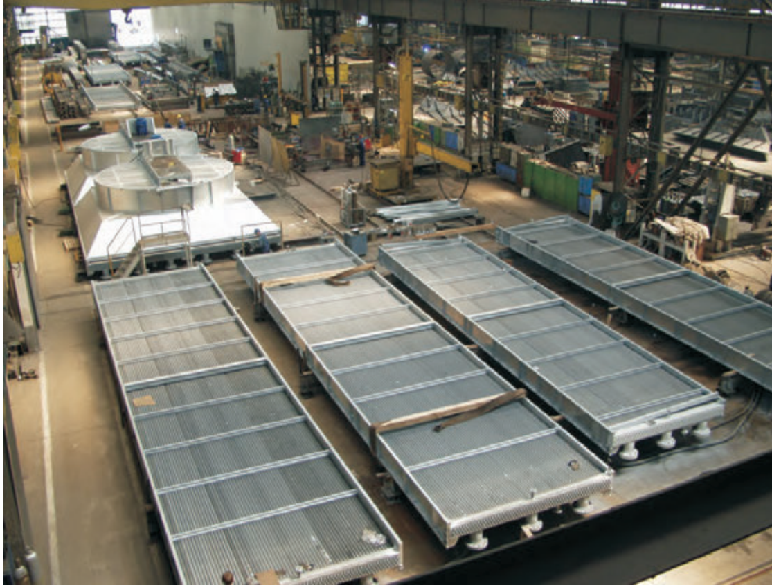
Finned tubes applied in air cooler tube bundle
