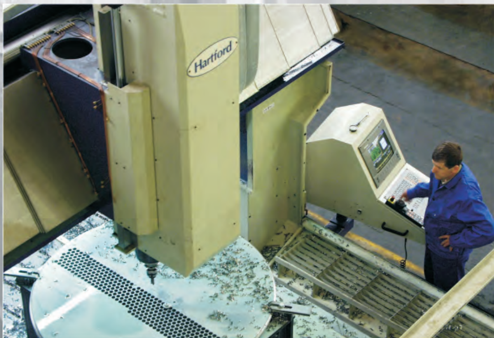
Drilling of heat exchanger tube sheet
