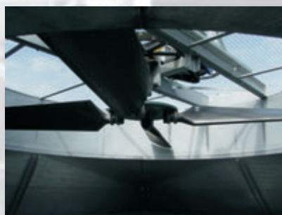
Fans installed in natural gas air coolers
