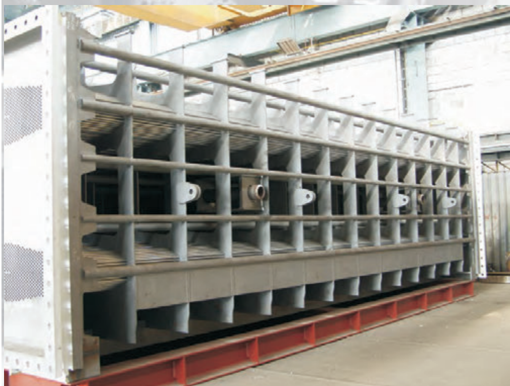
Assembly of turbine steam condenser
