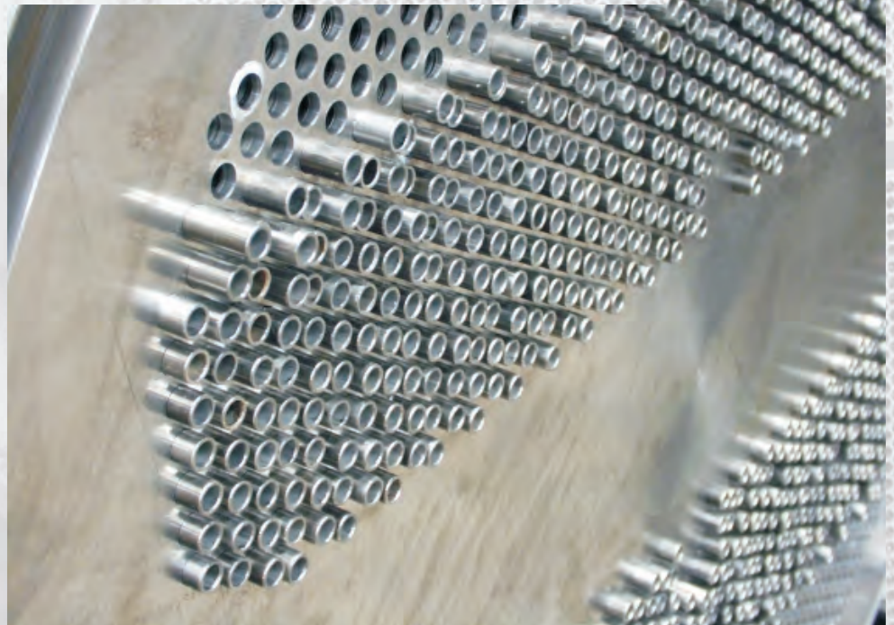
Putting of tube bundle into heat exchanger shell
