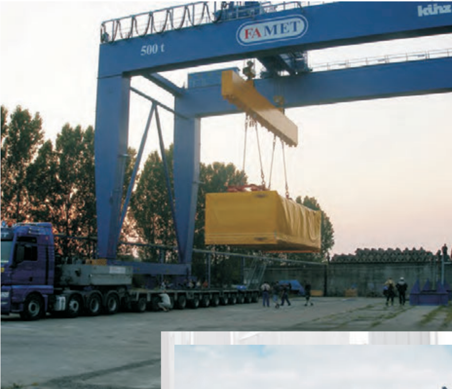
Gantry crane with lifting capacity of 500 tons
