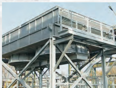
Trial assembly test of air cooler
