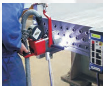
Orbital welding of tubes to header tube sheet through plug holes
