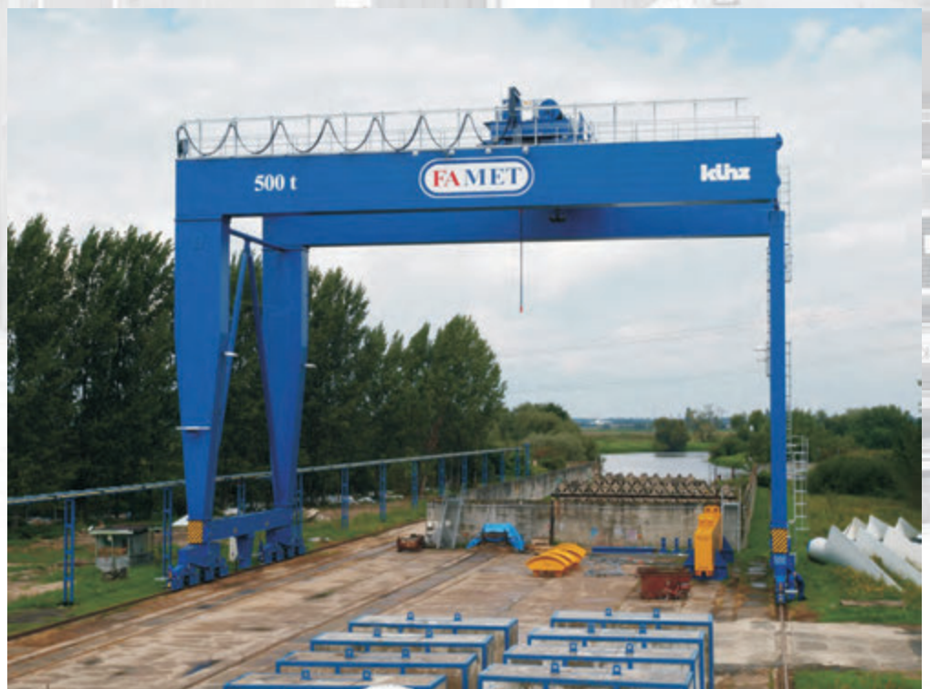
Gantry crane with lifting capacity of 500 tons
