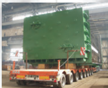
Assembly and transport of steam condenser
