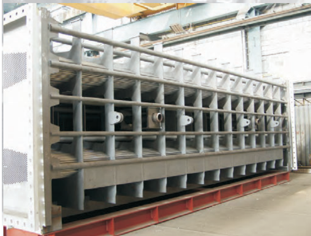
Assembly of turbine steam condenser
