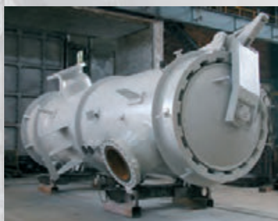
Assembly of gas filters
