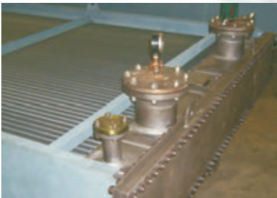
Water pressure test of tube bundle
