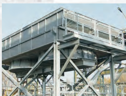
Trial assembly test of air cooler
