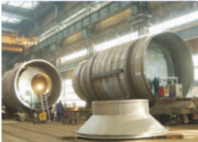
Assembly of evaporator
