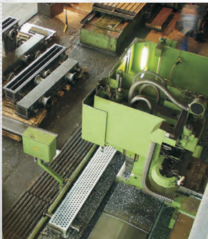
Welding of header by means of double-head welding machine
