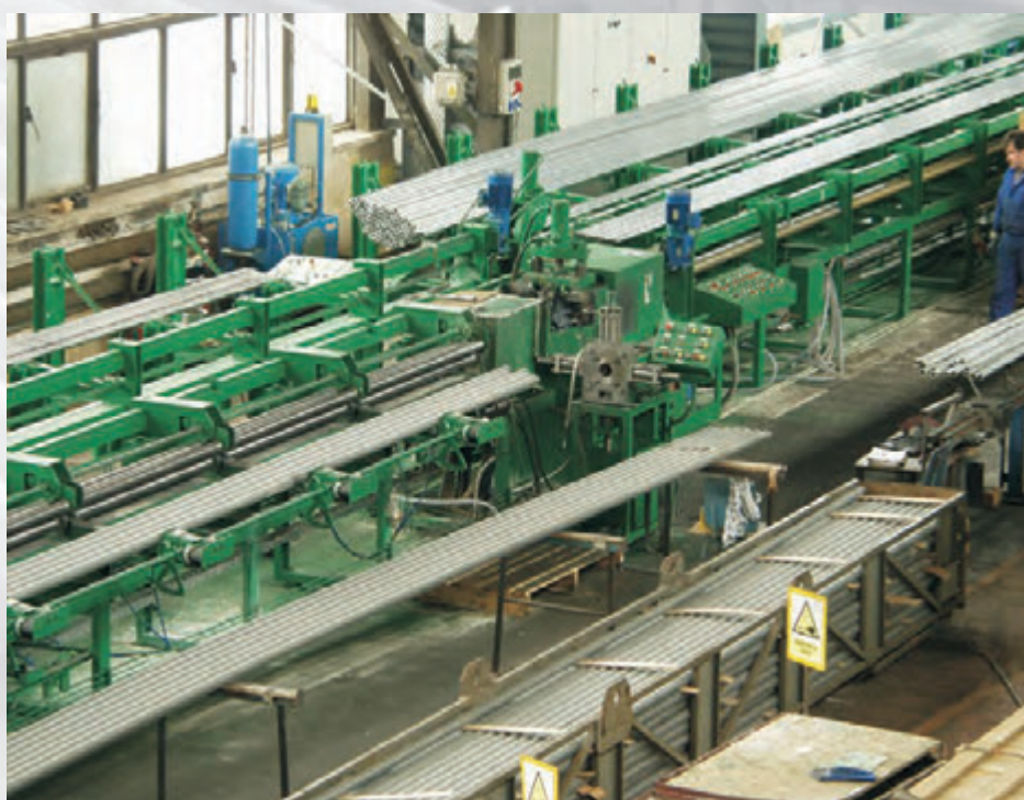
Machine for finning of tubes (length: 15.5 m.)
