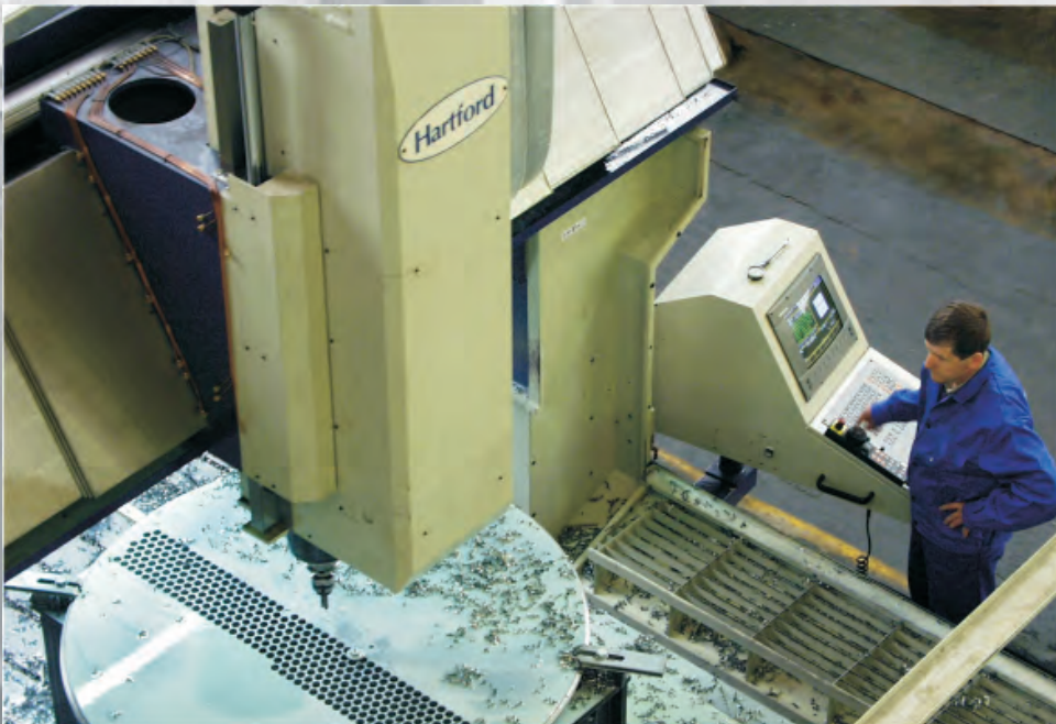
Drilling of heat exchanger tube sheet
