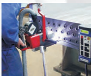
Orbital welding of tubes to header tube sheet through plug holes
