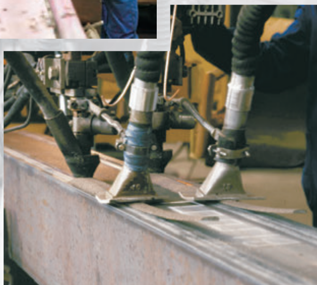
Welding of header by means of double-head welding machine
