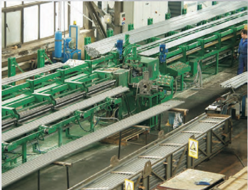
Machine for finning of tubes (length: 15.5 m.)
