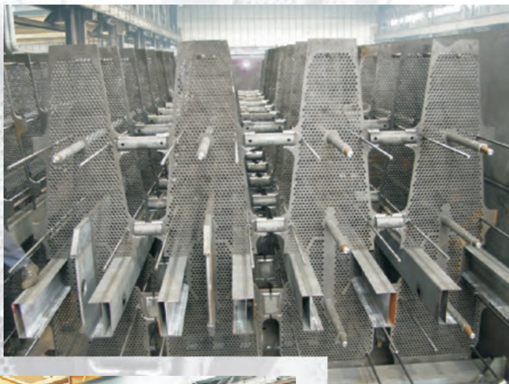
Assembly of turbine steam condenser
