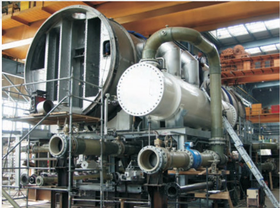
Evaporator of sea water desalination system during trial assembly
