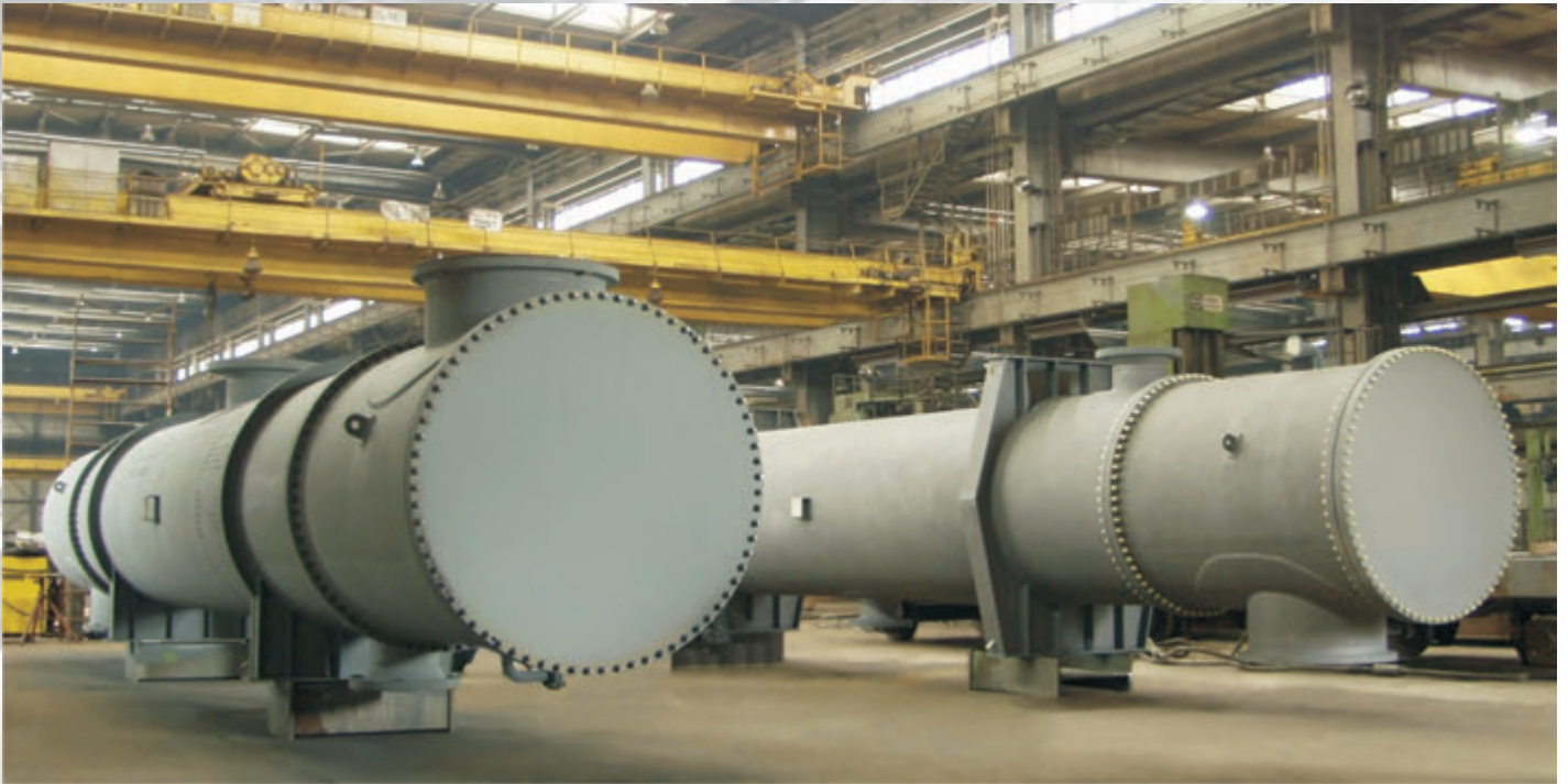
Battery of shell & tube heat exchangers in solar power plant
