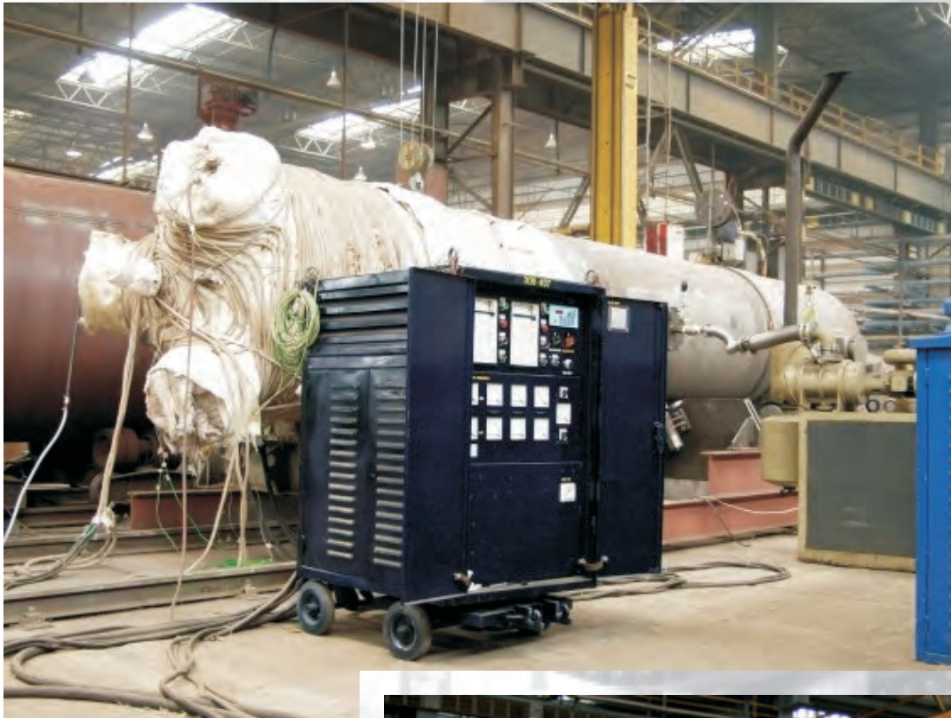
Heat treatment of high-pressure regenerative preheaters after welding
